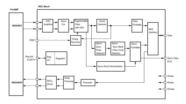
Figure 4.4 Read/write circuit block diagram
